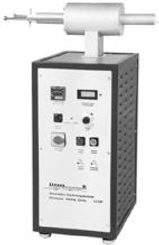
Figure 4: microwave heating chamber MEK 1,2 kW
