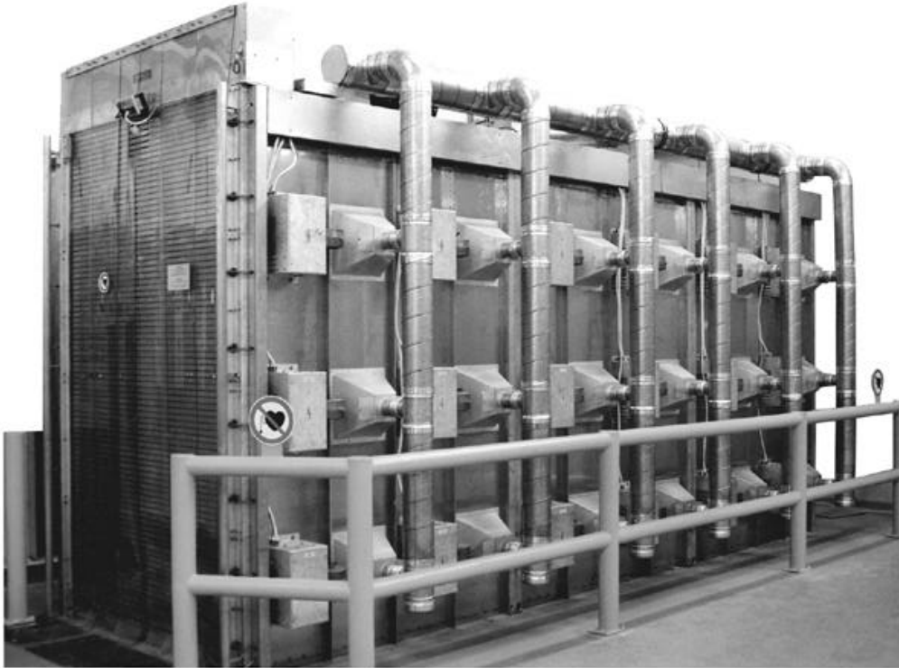
Figure 2: microwave chamber drier, chamber size 21 m 3 , 30 kW
