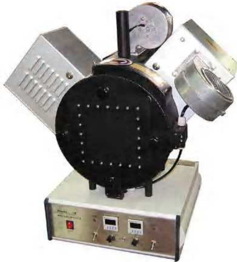
Figure 8: microwave dual frequency furnace, 800 W/2.45 GHz and 600 W/5.8 GHz
