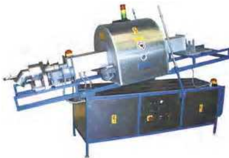
Figure 7: microwave rotary tube furnace MDRT 6,4 kW
