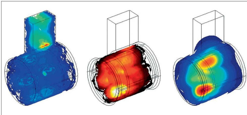
Fig. 14 Results of FEM-simulation: a) electrical field distribution, b) heating source density distribution and c) temperature distribution [4]
