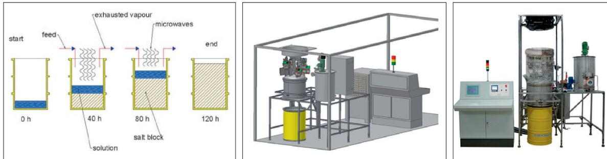
Fig. 6 Schematic diagram of MIDD-process (l.) and new MIDD prototype (r.)
