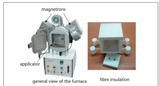
Fig. 8 Microwave laboratory furnace MKE-1,6
