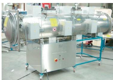
Fig. 5 Microwave chamber dryer MKST-9,6 200/2500
