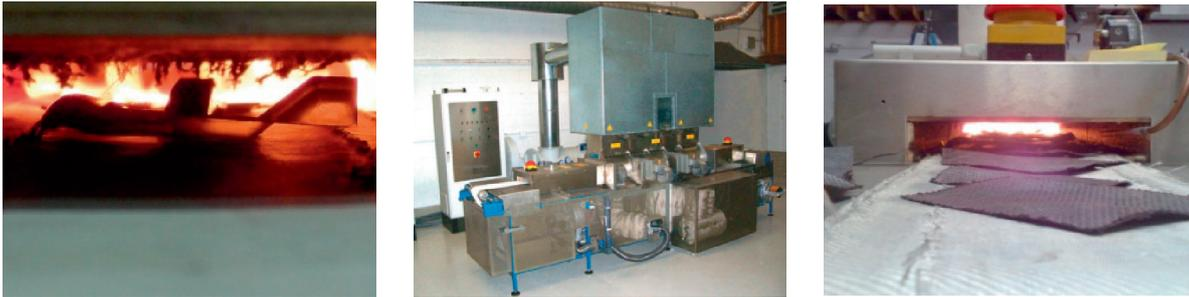
Fig. 12 Recycling of carbon fibres (l. and r.) and microwave hybrid continuous belt furnace (middle)
