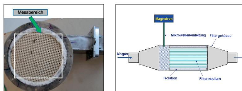
Fig. 13 Experimental setup (rear side) and test assembly for experimental validation of the 3D-FEM-simulation [4]
