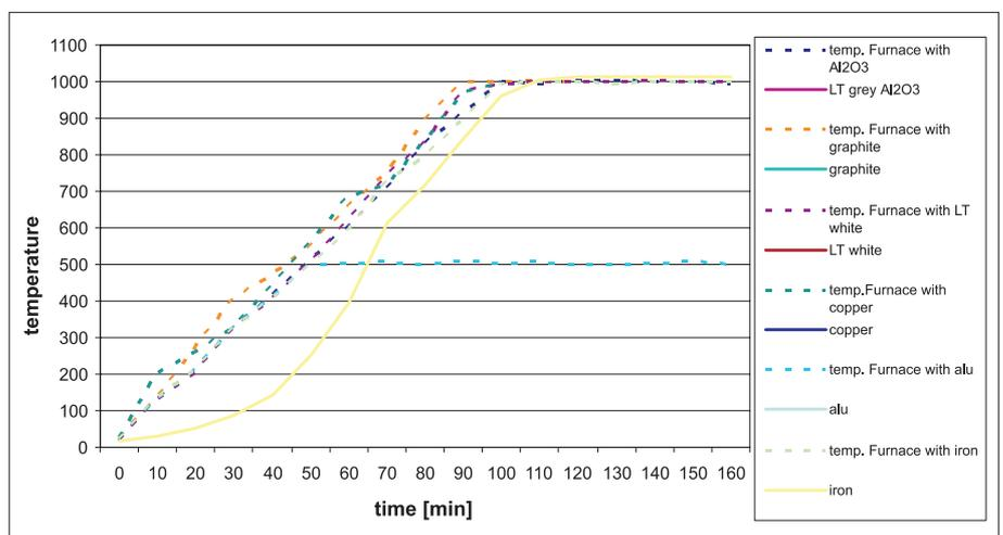
Fig. 9: Temperature process of different materials
