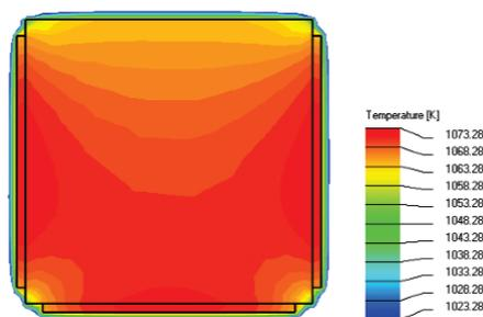
Fig. 10: Temperature distribution in the KS 80 S
