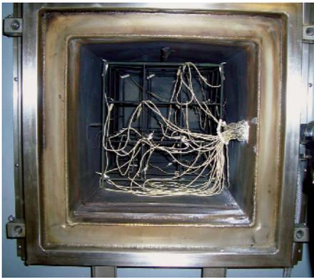
**Fig. 2:** Symmetrical installation of auxiliary grid in the chamber
