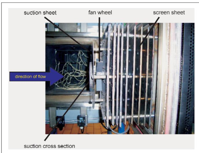
**Fig. 3:** Structure of revolution ventilator
