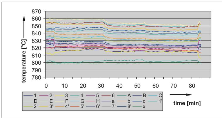
Fig. 6: Argon atmosphere, T = 800 °C, fan impeller 1, diameter 140 mm
