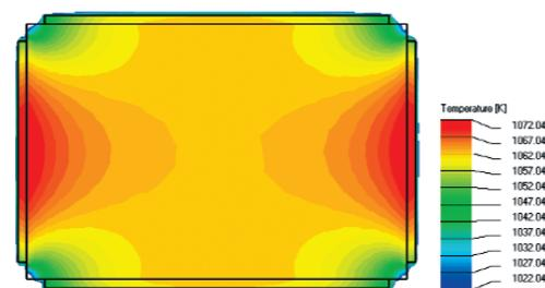
Fig. 11: Temperature distribution in the VMK 135 S
