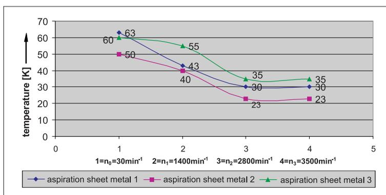
**Fig. 5:**  $dT/dt$  as function of suction metal sheet at various rotaries
