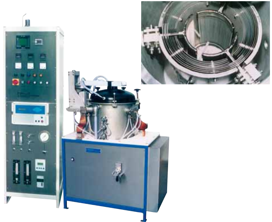
Fig. 7: Cold wall furnace KKV 140/270/2,000 up to 2,200°C. Toploader with tungsten mesh heater, turbomolecular pump up to 10 -5 mbar, gas supply and burning device for hydrogen
