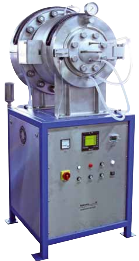
Fig. 6: High pressure furnace up to 1,000°C. Operation under pure oxygen up to 100 bar. Heated with molybdenum-disilicide. For development of High-Temperature Superconductiv materials (HTSC)
