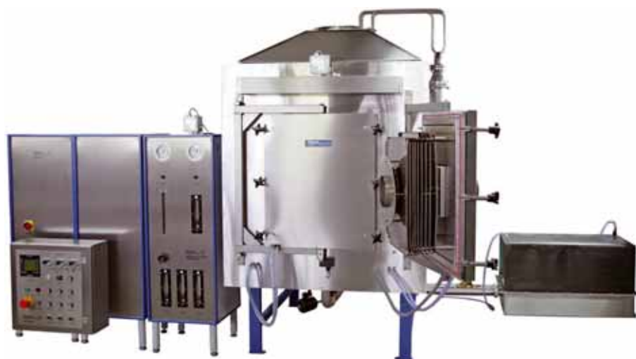
Fig. 3: Fibre insulated gastight furnace KF-240 S up to 1,200°C for reduction and sintering of precious metall pellets under hydrogen. Gas recooling by gas/water- heat exchanger for fast cooling. Furnace prepared for clean room installation
