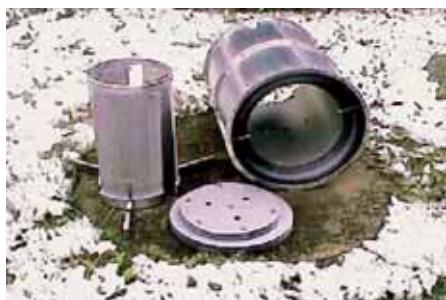
Fig. 8: Mesh heater with radiation screens for T_{max} 2,300°C
