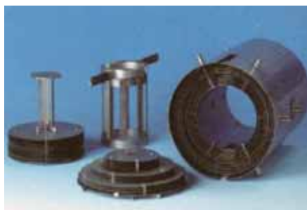
Fig. 9: Strip heater with radiation screens and working plate for T_{max} 3,000°C
