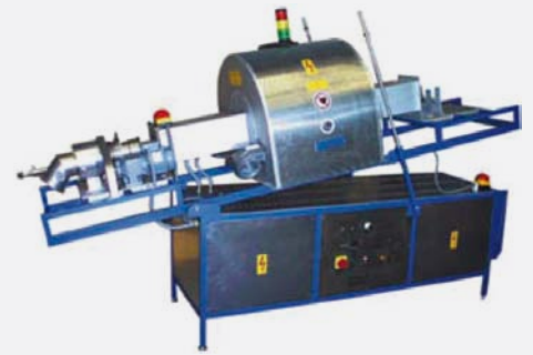
Fig. 4: Gas and vacuum sealed microwave rotary furnace for CVD process
