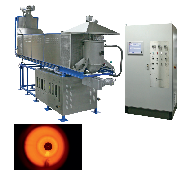
Fig. 4 FDHK-3-140/2200/1100 rotary tube furnace for uranium oxide reduction: view of hot zone of the furnace tube
